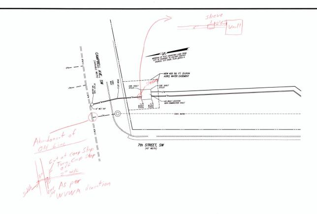
Contractor's original hard copy red-line annotated as-built documents. Contractor shall provide a statement and signature on this set of documents certifying that the work was done in accordance with these documents, with reasonable accuracy, and that any deviations have been red-line annotated or otherwise captured in change order documentation.
