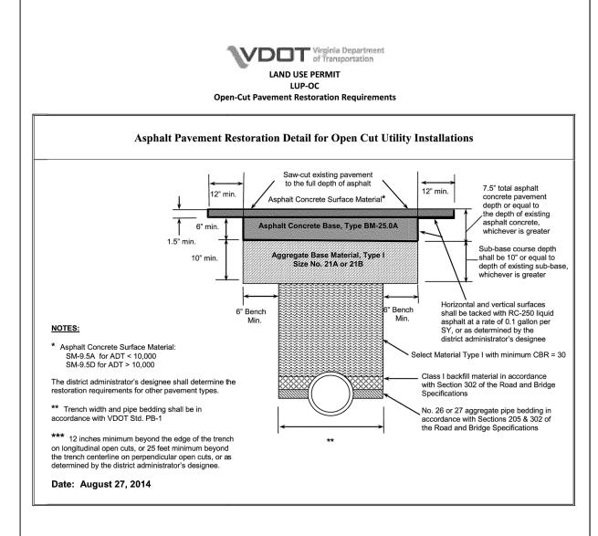
1. ALL PAVEMENT RESTORATION WITHIN THE RIGHT-OF-WAY SHALL BE COMPLETED PER THE REQUIREMENTS OF THIS DETAIL, AND AS SHOWN ON THE PLANS.
