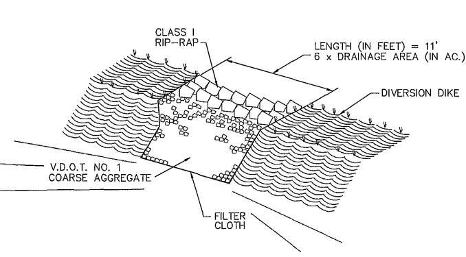
COARSE AGGREGATE SHALL BE VDOT #3, #357, OR #5
