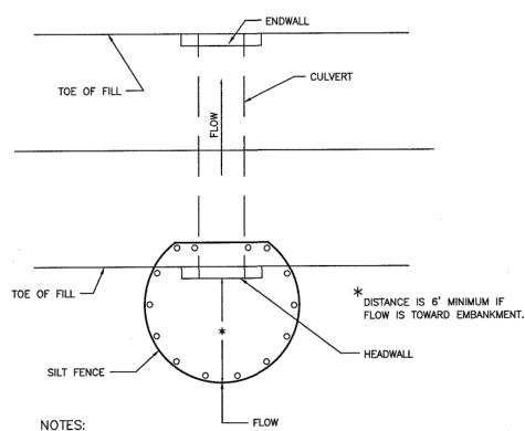
If silt fence culvert inlet protection is not sufficient due to expected high velocity of flow, contractor shall install optional stone and inlet sediment trap protection per STD. & SPEC. 3.08.
