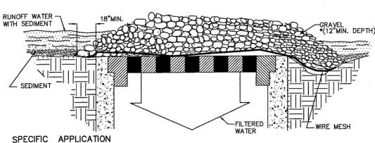
This method of inlet protection is applicable where heavy concentrated flows are expected, but not where ponding around the structure might cause excessive inconvenience or damage to adjacent structures and unprotected areas.
