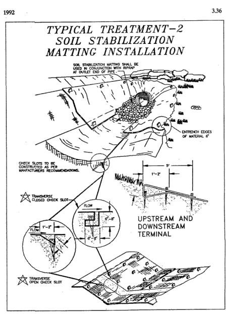
Plate 3.36-4 Source: VDOT Road and Bridge Standards NOTE: MATTING SHALL BE INSTALLED AND ANCHORED IN ACCORDANCE WITH MANUFACTURER'S INSTRUCTIONS.
