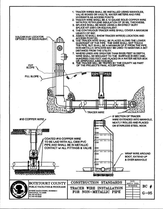
\_ocator Wire Shall Be Installed From The Watermain To The Meter Box.
