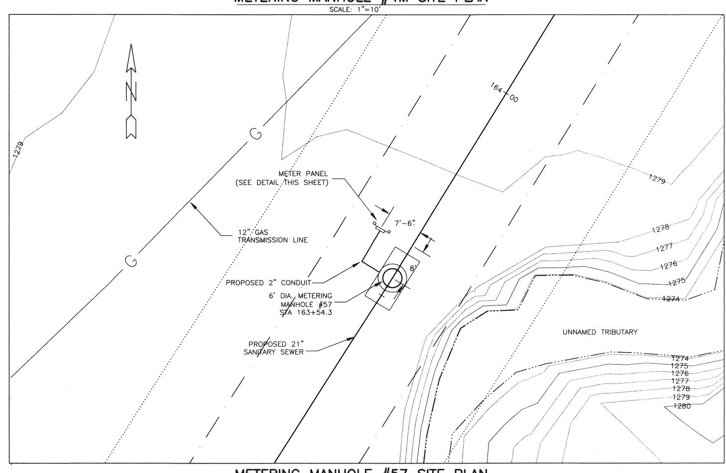
METERING MANHOLE #57 SITE PLAN SCALE: 1"=10"
