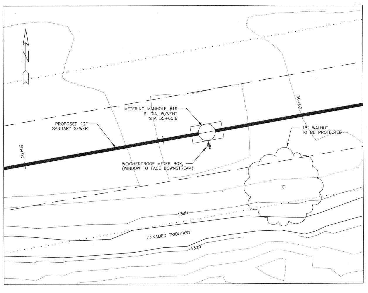
METERING MANHOLE #19 SITE PLAN
