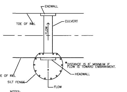
SILT FENCE CULVERT INLET PROTECTION
