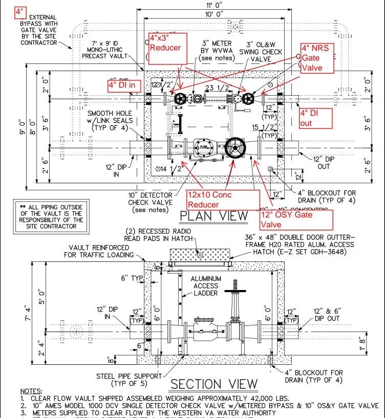
4. 3" CLAVAL #585LW OUTSIDE LEVER & WEIGHT SWING CHECK VALVE
