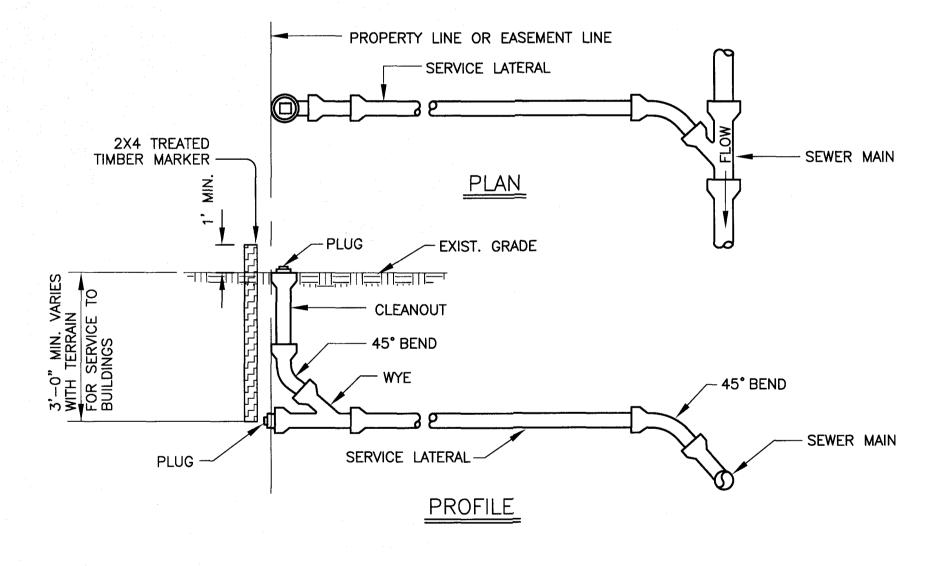
FOR RESIDENTIAL CONNECTIONS, LATERAL PIPES SHALL BE 4" DIA. PVC-SDR35 OR SCH. 40. FOR COMMERCIAL CONNECTIONS, THE LATERAL SIZE SHALL BE SPECIFIED ON THE PLANS BY THE ENGINEER.
