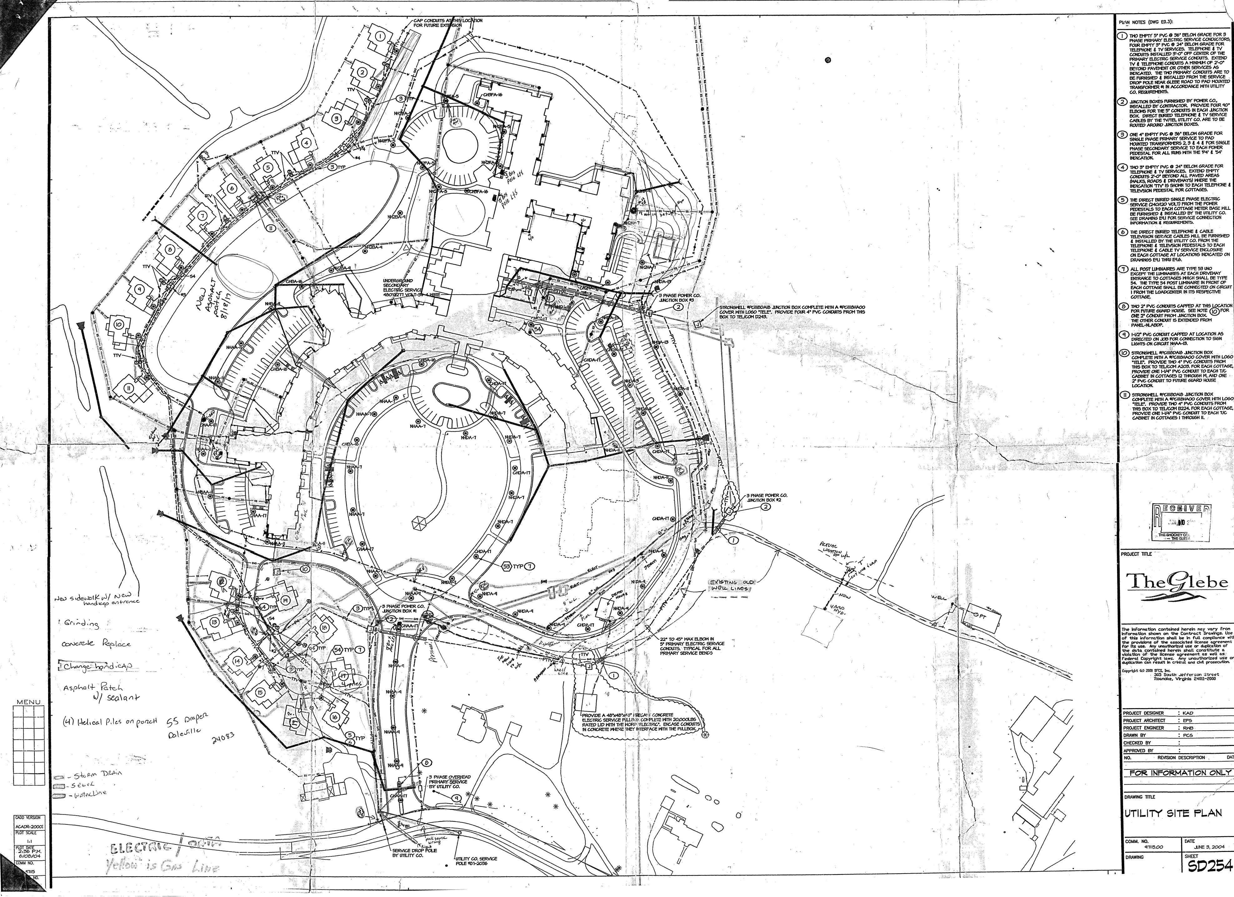
PHASE PRIMARY ELECTRIC SERVICE CONDUCTORS FOUR EMPTY 3" PVC @ 24" BELOW GRADE FOR TELEPHONE & TV SERVICES. TELEPHONE & TV CONDUITS INSTALLED 3'-0" OFF CENTER OF THE PRIMARY ELECTRIC SERVICE CONDUITS. EXTEND TY & TELEPHONE CONDUITS A MINIMUM OF 2'-0" BEYOND PAVEMENT OR OTHER SERVICES AS INDICATED. THE TWO PRIMARY CONDUITS ARE TO BE FURNISHED & INSTALLED FROM THE SERVICE DROP POLE NEAR GLEBE ROAD TO PAD MOUNTED TRANSFORMER # IN ACCORDANCE WITH UTILITY
