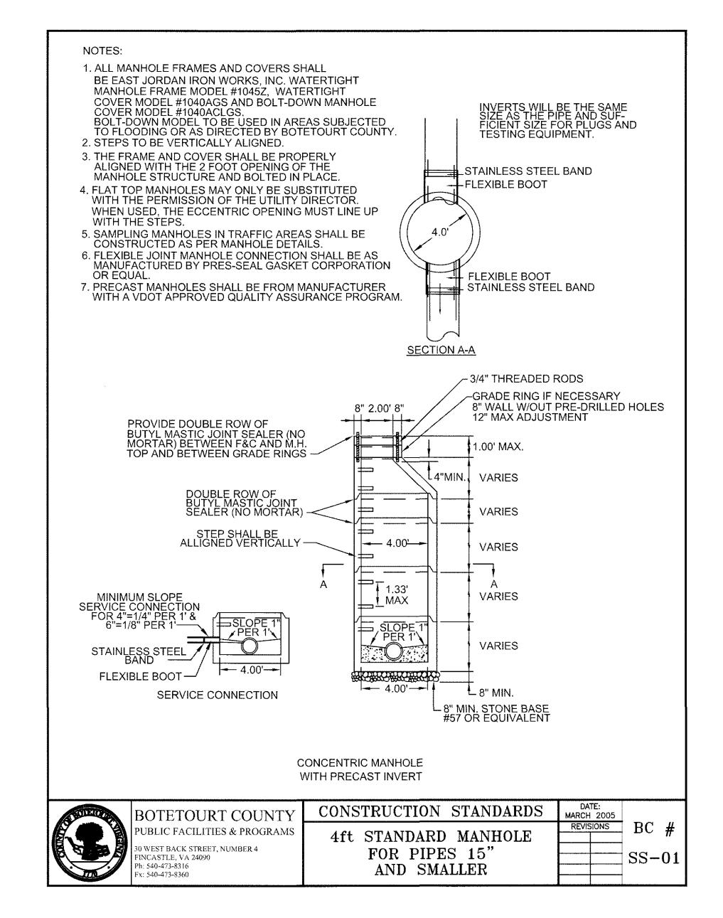
NOTE: SANITARY DROP CONNECTIONS, WHERE INDICATED, PER VDOT SMH-I DETAIL.
