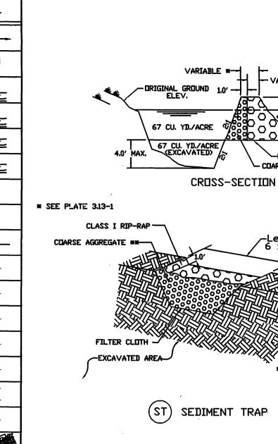
6 x Drainage Area (ac.) \*\* COARSE AGGREGATE SHALL BE VDUT #3,#357 0F#5
