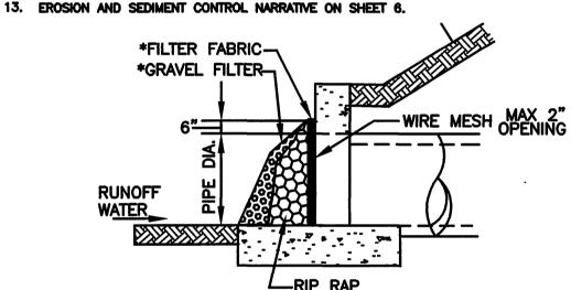
INLET PROTECTION DETAIL FOR SEDIMENT TRAP #2
