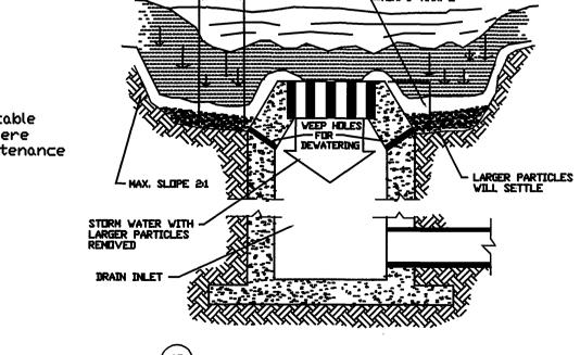
EXCAVATED DROP INLET SEDIMENT TRAP
