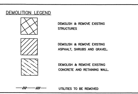
CONTRACTOR TO COORDINATE WITH THE APPLICABLE UTILITY COMPANY WHEN REMOVING AND / OR RELOCATING UTILITIES.
