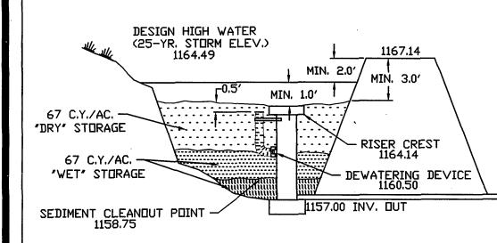
DESIGN ELEVATIONS WITHOUT EMERGENCY SPILLWAY (RISER PASSES 25-YR. EVENT)
