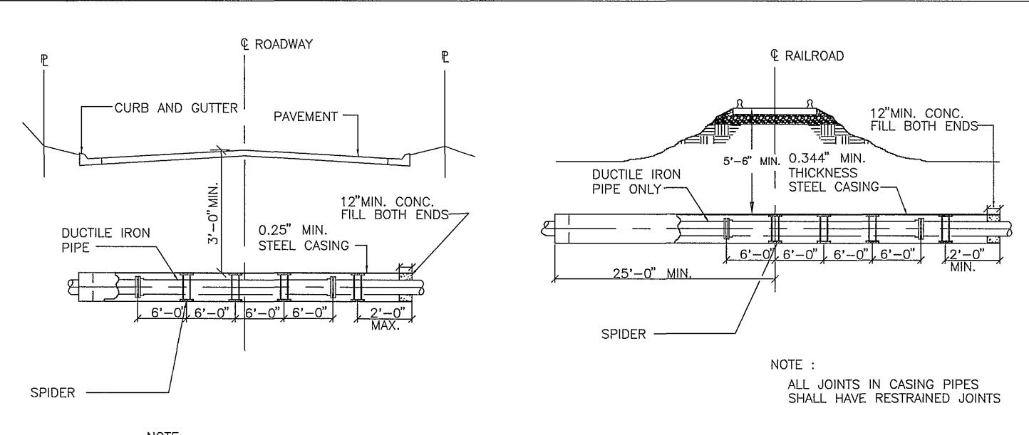
NOTE: STEEL CASING TO EXTEND TO BACK OF CURB OR MIN. 3'-0" BEYOND EDGE OF PAVEMENT
