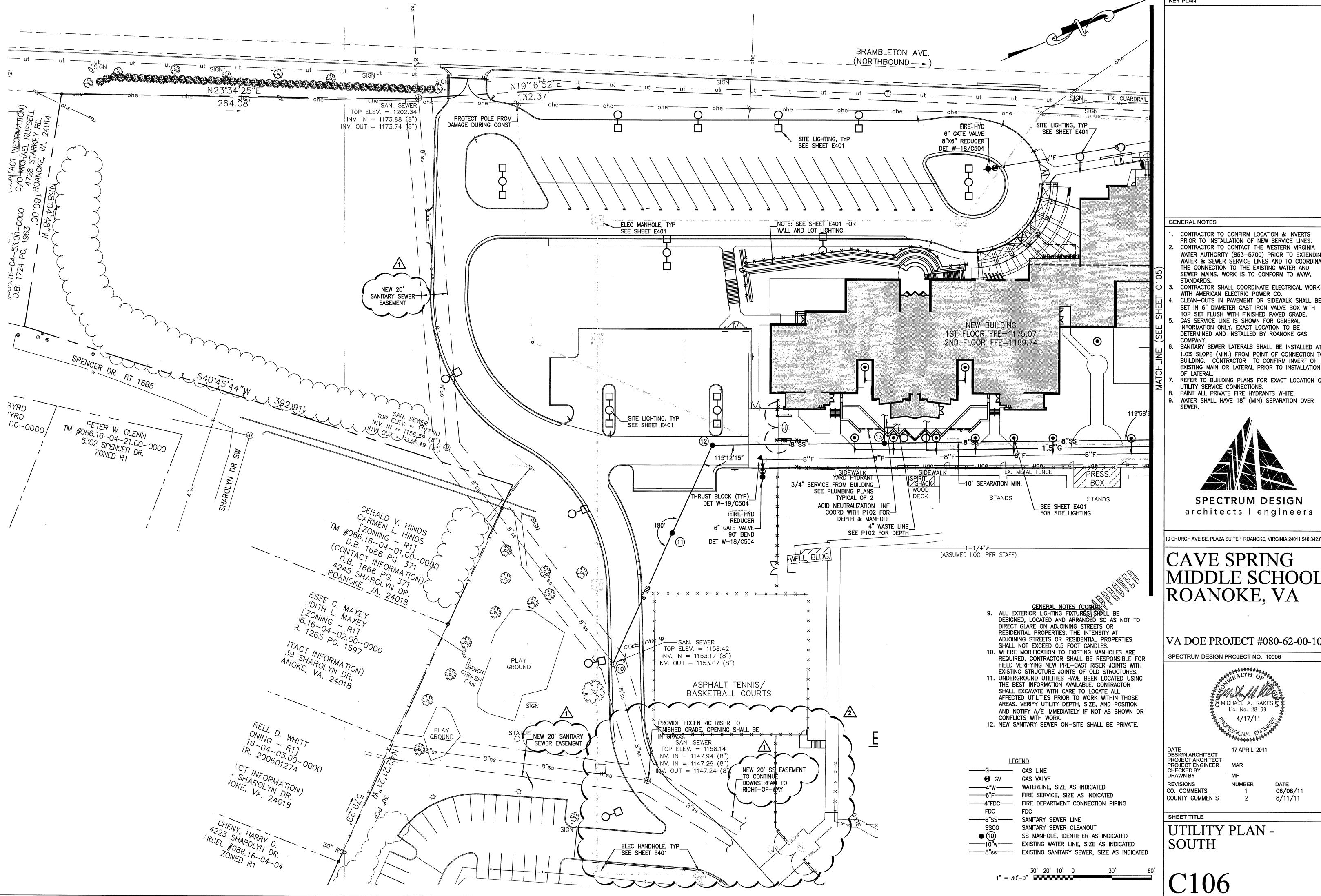
PRIOR TO INSTALLATION OF NEW SERVICE LINES. CONTRACTOR TO CONTACT THE WESTERN VIRGINIA WATER AUTHORITY (853-5700) PRIOR TO EXTENDING WATER & SEWER SERVICE LINÉS AND TO COORDINATE THE CONNECTION TO THE EXISTING WATER AND SEWER MAINS. WORK IS TO CONFORM TO WVWA
