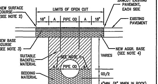
NOTE 3. COMPACTED ASPHALT CONCRETE BASE COURSE, 3" OF TYPE BM-2
