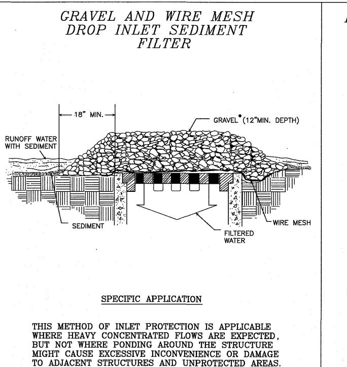
\* GRAVEL SHALL BE VDOT #3, #357 OR #5 COARSE AGGREGATE.
