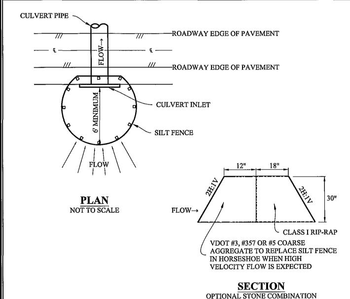
1. The height of the silt fence (in front of the culvert opening) shall be a minimum of 16 in. and shall not exceed 34 in.
