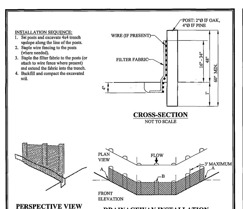
NOT TO SCALE Synthetic filter fabric shall be a pervious sheet of propylene, nylon, polyester or ethylene yarn and shall be certified by the manufacturer or supplier as conforming to the requirements noted in VESCH Table 3.05-B, latest edition. The filter fabric shall be purchased in a continuous roll cut to the length of the barrier to avoid the use of joints. When joints are unavoidable, filter cloth shall be spliced together only at a support post, with a minimum 6-inch overlap,
