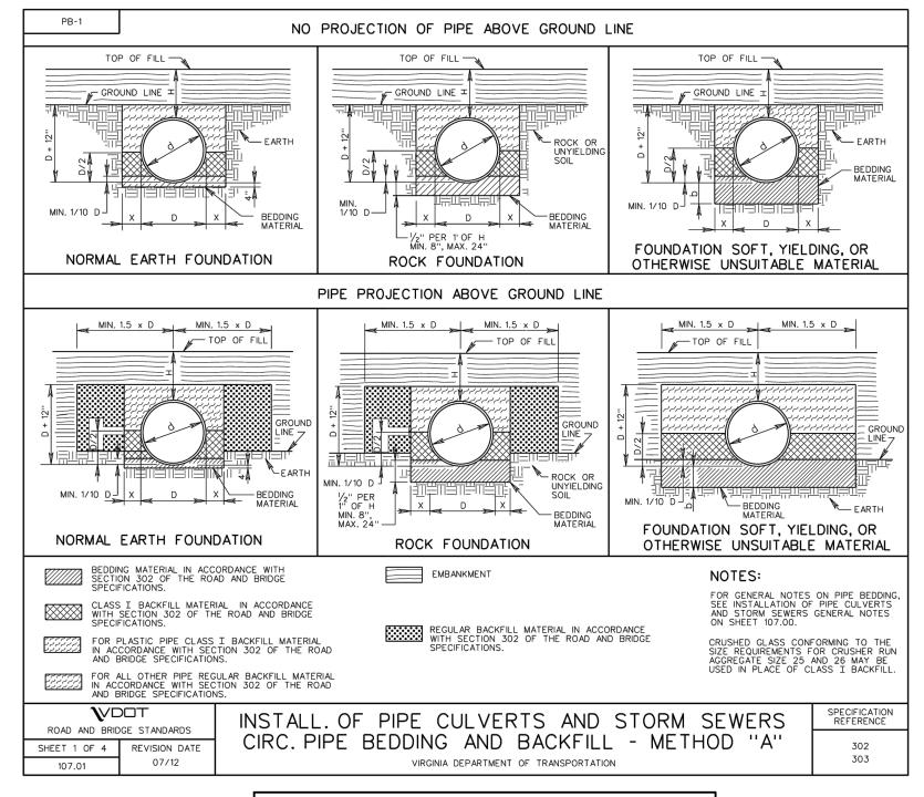
NOTE: CLASS I BACKFILL SHALL BE CRUSHER RUN AGGREGATE SIZE NO. 25 OR 26, AGGREGATE BASE MATERIAL SIZE 21A OR 21B, FLOWABLE FILL, OR CRUSHED GLASS CONFORMING TO THE SIZE REQUIRED FOR CRUSHER RUN AGGREGATE SIZE 25 AND 26.
