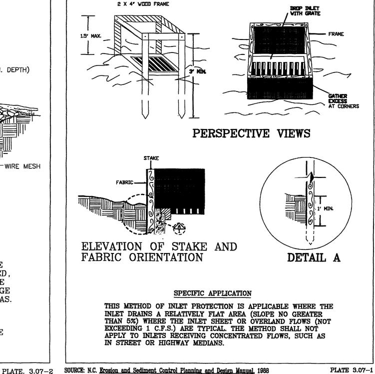
SILT FENCE DROP INLET
