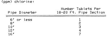
or the number of tablets equal to 0.0012d L rounded to the next higher integer, where d is the inside diameter, in inches and L is the length of the pipe section, in feet. Use of the continuous feed or slug method of disinfecting may only be used to re-chlorinate a water pipe after the initial disinfection or in other specific cases approved by the Design Engineer. When filling the pipeline for disinfection, the rate of filling must result in a velocity of less than 1 ft./sec.
