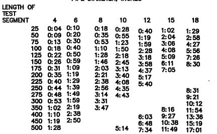
SHOULD THE 1.0 PSI DROP OCCUR IN LESS TIME THAN THAT SPECIFIED IN THE TABLE, THE SEWER SEGMENT SHALL HAVE FAILED. IF THE TIME REQUIRED FOR THE PRESSURE TO DROP 1.0 PSI IS GREATER THAN THAT SHOWN IN THE TABLE, THE SEWER SEGMENT SHALL HAVE PASSED.
