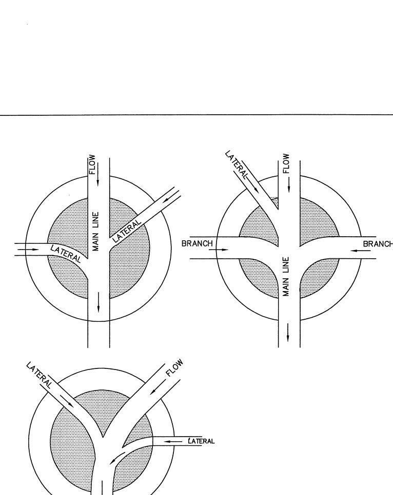
THE INVERT CHANNELS SHALL BE FORMED WITH CONCRETE AS SHOWN AND SHALL BE SMOOTH AND SEMI-CIRCULAR IN SHAPE, CONFORMING TO THE INSIDE OF THE ADJACENT SEWER SECTION. CHANGES IN THE DIRECTION OF FLOW SHALL BE MADE WITH A SMOOTH CURVE OF AS LARGE A RADIUS AS SIZE OF MANHOLE WILL PERMIT.
