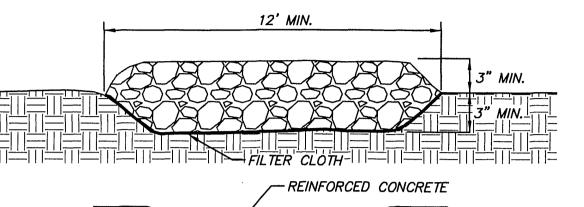
DRAIN SPACE-WASH RACK DETAIL AS REQUIRED BY LOCAL AUTHORITY AND BY SPECIFIC CONDITIONS.
