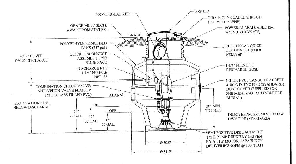
E-ONE GRINDER PUMP STATION, MODEL NO. 1012s-73
