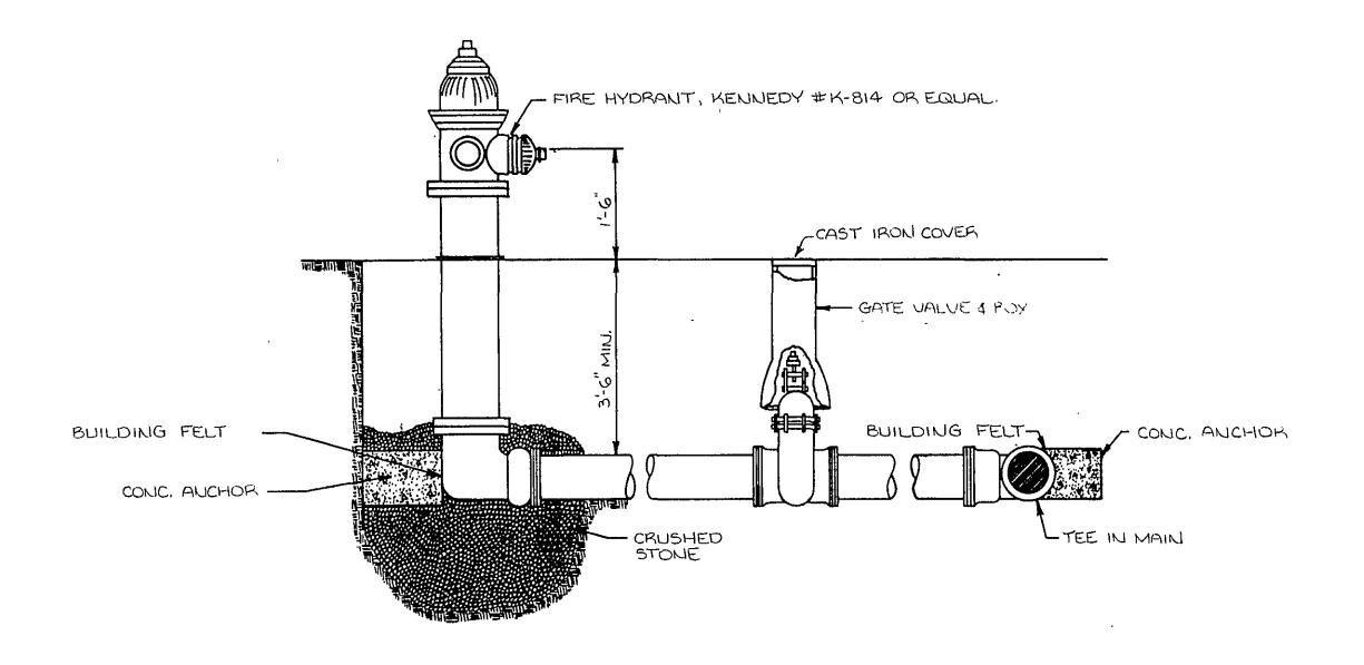
TYPICAL GATE VALVE INSTALLATION 301.1
