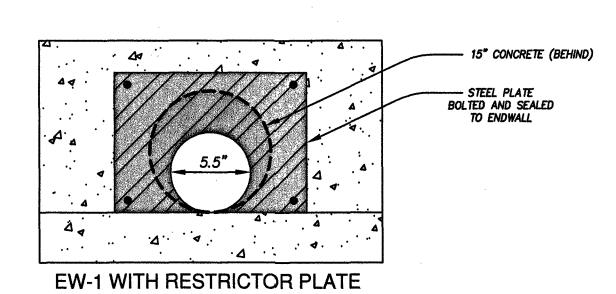
NO SCALE NOTE: EW-1 WITH RESTRICTOR PLATE REQUIRES INSTALLATION
