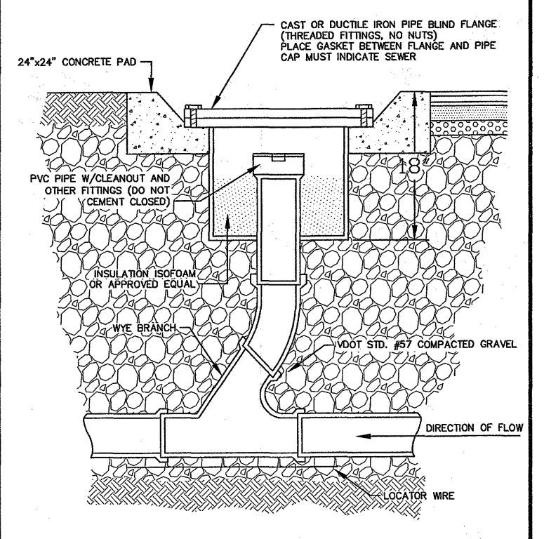
PVC PIPE TO BE OF AWWA C-900, SDR-21, CLASS 100 SPECIFICATION
