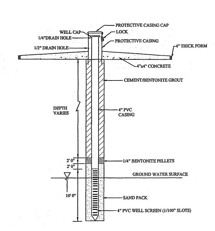
GROUND WATER MONITORING WELL DETAIL
