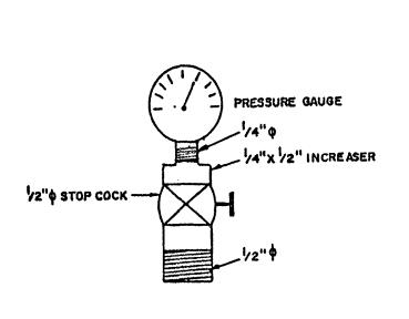
PORTABLE DRAWDOWN GAUGE ASSEMBLY - DETAIL
