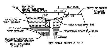
DESIGN ELEVATIONS WITH EMERGENCY SPILLWAY
