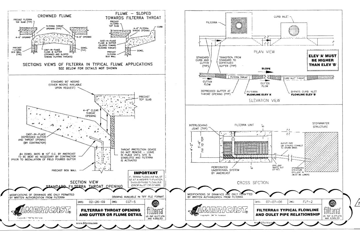
TREE BOX STORMWATER FILTER SPECIFICATIONS
