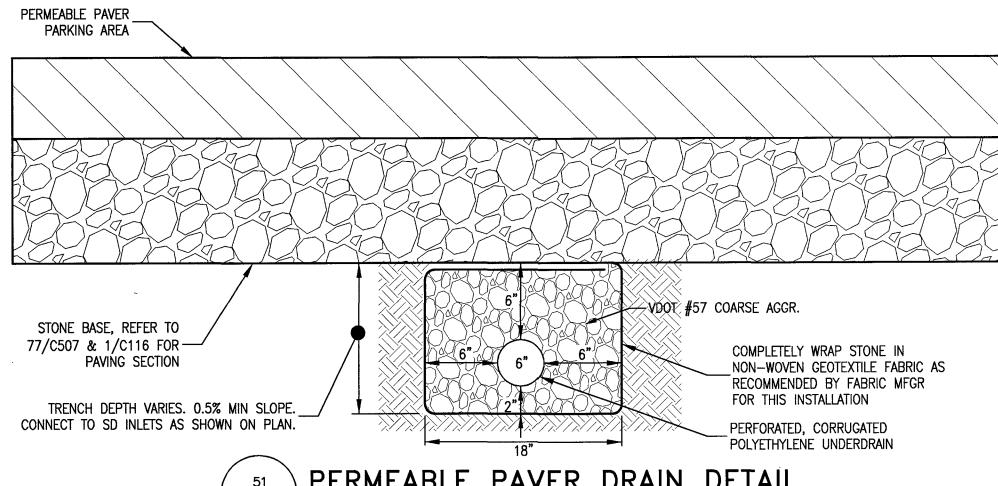
PERMEABLE PAVER DRAIN DETAIL
