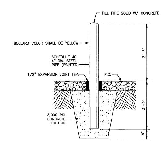
STEEL PIPE BOLLARD DETAIL NO SCALE
