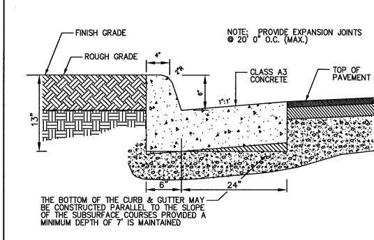
G.C. SHALL BE RESPONSIBLE FOR OBTAINING ADEQUATE SUB-GRADE COMPACTION.
