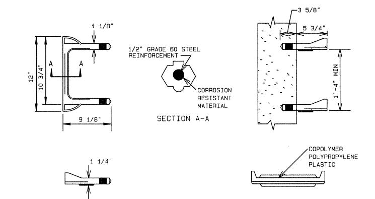
STEPS WILL BE REQUIRED IN ALL STRUCTURES WITH A DEPTH OF 4'-0" OR GREATER UNLESS ETHERWISE NOTED ON THE PLANS.
