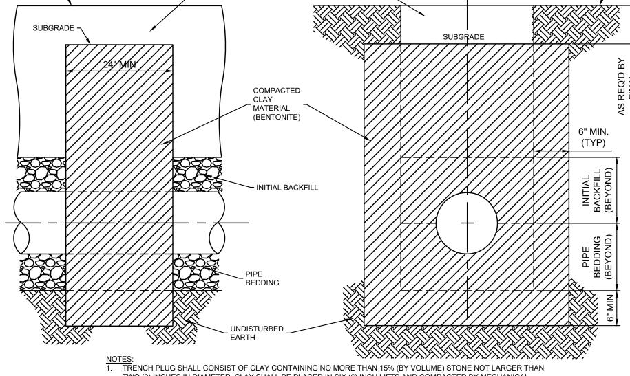
TWO (2) INCHES IN DIAMETER. CLAY SHALL BE PLACED IN SIX (6) INCH LIFTS AND COMPACTED BY MECHANICAL TAMPER TO NOT LESS THAN 95% OF MAXIMUM DENSITY AT OPTIMUM MOISTURE CONTENT. 2. HEIGHT OF TRENCH PLUG TO EXTEND 1' FROM FINAL GRADE.
