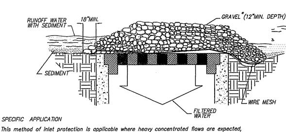
but not where ponding around the structure might cause excessive inconvenience or damage to adjacent structures and unprotected areas.
