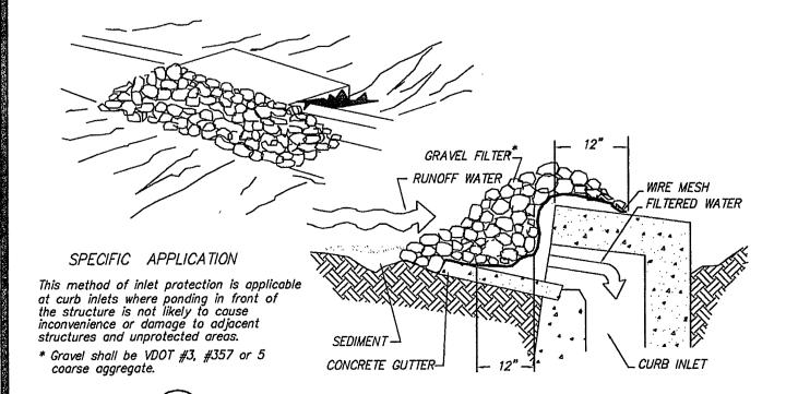
(IP) GRAVEL CURB INLET SEDIMENT FILTER
