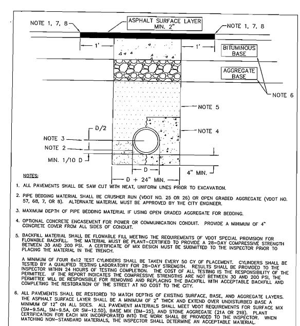
'. THE REPAIR SHALL BE RECTANGULAR AND SAW CUT IN STRAIGHT, UNIFORM LINES THAT ARE ALIGNED WITH THE STREET CENTERLINE. WHEN EDGES OF PAVEMENT HAVE BEEN UNDERMINED, PAVEMENT SHALL BE REMOVED TO A NEAT LINE 12" BEYOND THE UNDERMINED AREA. THE FINISHED PATCH SURFACE SHALL BE WITHIN 1/4 INCH AT ANY POINT ACROSS THE PATCH AS IT RELATES TO THE SURROUNDING STREET SURFACE.
