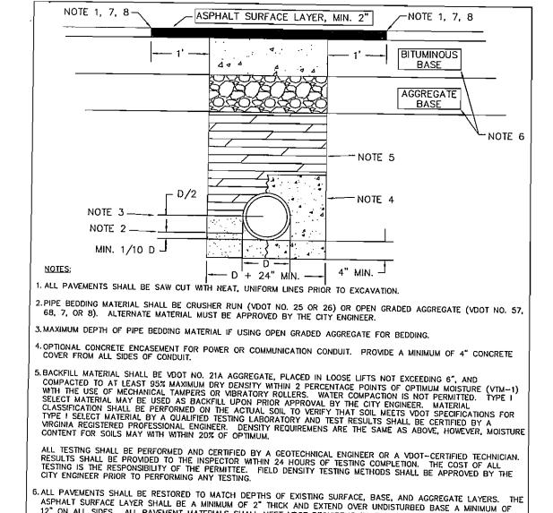
12" ON ALL SIDES. ALL PAVEMENT MATERIALS SHALL MEET VOOT REQUIREMENTS FOR SURFACE MIX (SM-9.5AL,
