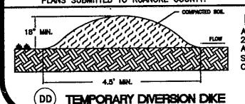
ALL DIVERSION DIKES THAT EXCEED 2% IN SLOPE MUST BE STABILIZED IN ACCORDANCE WITH VESCH STD. & SPEC. 3.17 (STORMWATER CONVEYANCE CHANNEL.
