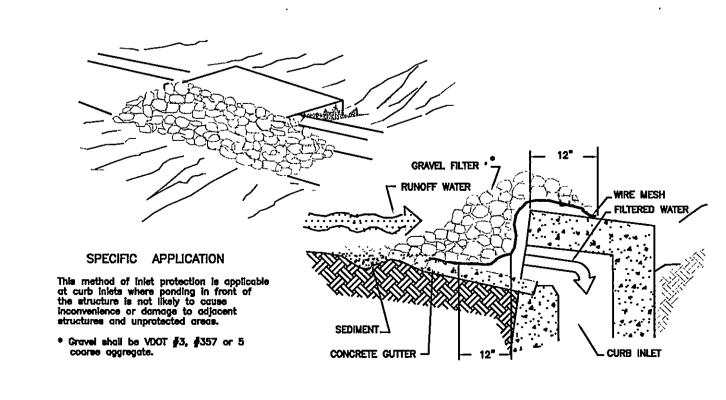
P GRAVEL AND WIRE MESH DROP INLET SEDIMENT FILTER
