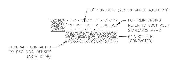
G.C. SHALL BE RESPONSIBLE FOR OBTAINING ADEQUATE SUB-GRADE COMPACTION.
