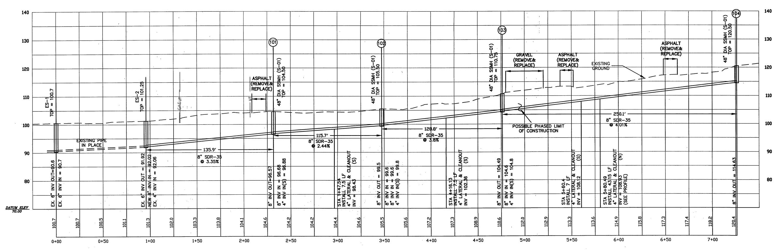
SANITARY SEWER LINE EXTENSION PROFILE - BROADLAWN RD FROM SANITARY SEWER MANHOLE ES-1 TO ES-2 TO 101 THROUGH 104
