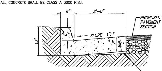
BOTTOM OF THE CURB & GUTTER -MAY BE CONSTRUCTED PARALLEL TO THE SLOPE OF THE SUBBASE
