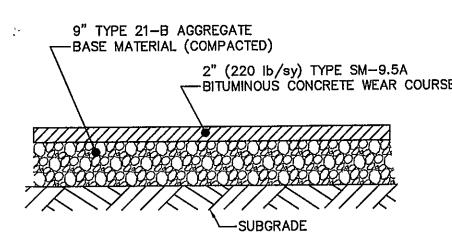
FOR AN EXCAVATED SUBGRADE: THE SUBGRADE AREA SHALL BE SCARIFIED TO A DEPTH OF 6 INCHES FOR A DISTANCE OF 2 FEET BEYOND THE PROPOSED EDGES OF THE PAVEMENT ON EACH SIDE. SUBGRADE MATERIAL SHALL BE COMPACTED AT OPTIMUM MOISTURE (±20%) TO THE REQUIREMENTS SET FORTH BY SEC. 305.03 OF THE VDOT ROAD AND BRIDGE SPECIFICATIONS
