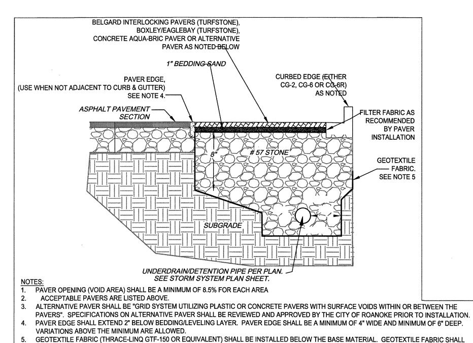
BE TURNED UP ON THE SIDES OF THE BASE LAYER. VARIATIONS BASED ON INSTALLATION RECOMMENDATIONS ARE ALLOWED.
