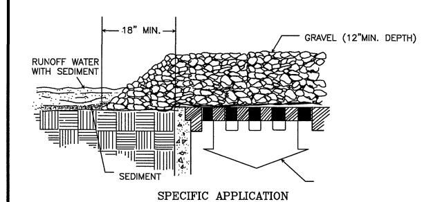
THIS METHOD OF INLET PROTECTION IS APPLICABLE WHERE HEAVY CONCENTRATED FLOWS ARE EXPECTED BUT NOT WHERE PONDING AROUND THE STRUCTURE MIGHT CAUSE EXCESSIVE INCONVENIENCE OR DAMAGE TO ADJACENT STRUCTURES AND UNPROTECTED AREAS
