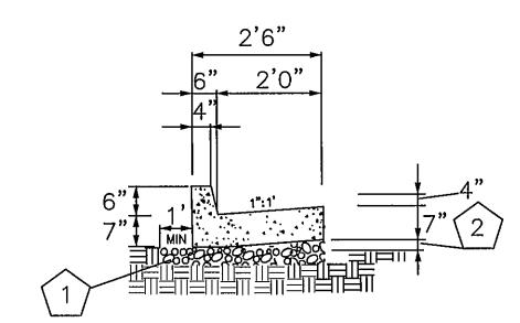
THE BOTTOM OF THE CURB AND GUTTER MAY BE CONSTRUCTED PARALLEL TO THE SLOPE OF SUBSURFACE COURSES PROVIDED A MINIMUM DEPTH OF 7" IS MAINTAINED.
