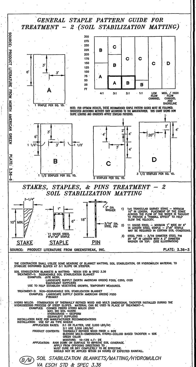
FOR THE PURPOSE OF THIS PROJECT, THE CONTRACTOR SHALL ANTICIPATE UTILIZATION OF SOIL STABILIZATION BLANKETS — TREATMENT 2, WITH STAPLE PATTERNS A & B FOR SLOPES.
