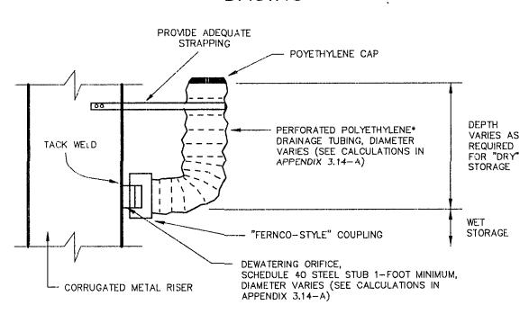
NOTE: WITH CONCRETE RISER, USE PVC SCHEDULE 40 STUB FOR DEWATERING ORIFICE
