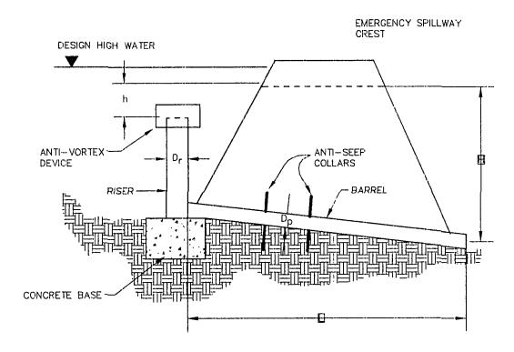
H = HEAD ON PIPE THROUGH EMBANKMENT h = HEAD OVER RISER CREST L = LENGTH OF PIPE THROUGH EMBANKMENT DD = DIAMETER OF PIPE THROUGH EMBANKMENT  $D_r = DIAMETER OF RISER$
