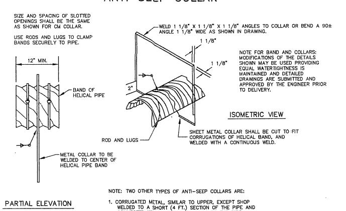
CONNECTED WITH CONNECTING BANDS TO THE PIPE.
