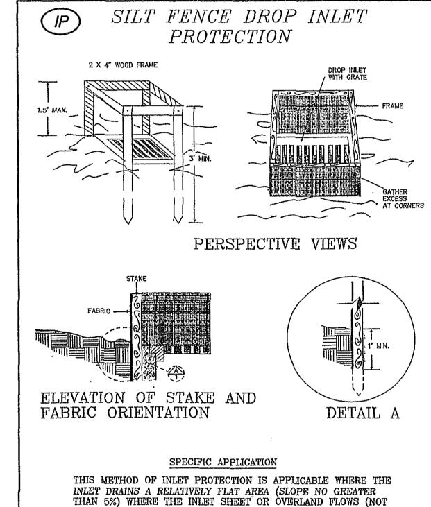
EXCEEDING 1 C.F.S.) ARE TYPICAL. THE METHOD SHALL NOT APPLY TO INLETS RECEIVING CONCENTRATED FLOWS, SUCH AS IN STREET OR HIGHWAY MEDIANS.
