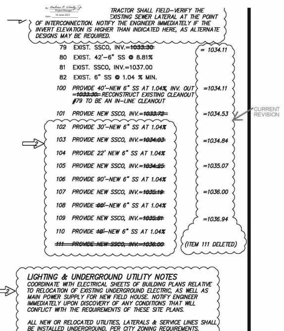
PATRICK HENRY FIELD HOUSE - FIELD REVISION TO PRIVATE SANITARY SEWER LATERAL REVISION REQUIRED DUE TO INVERT ELEVATION AT POINT OF INTERCONNECTION BEING 0.81 FEET HIGHER THAN ANTICIPATED. ALL SLOPES REMAIN PER PLAN, HOWEVER, THE POINT OF EXIT FROM THE BUILDING HAS BEEN REVISED TO THE PRACTICE FIELD SIDE DATE: 2020-12-23 PREPARED BY C.L. White - CWA SHEET 1 OF 2 (PORTION OF C-05)
